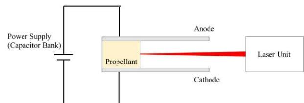
Figure 1. schematic of a LA-PPT
