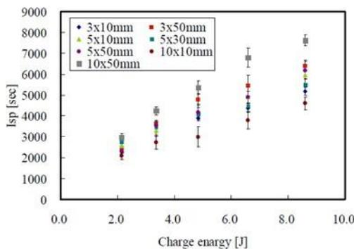
Figure 3. the various case of typical characteristics when the laser assisted PPT operated high specific impulse
