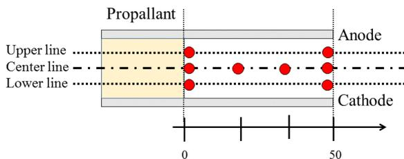
Figure 10. probe arrangements when we conduct experiment in the past
