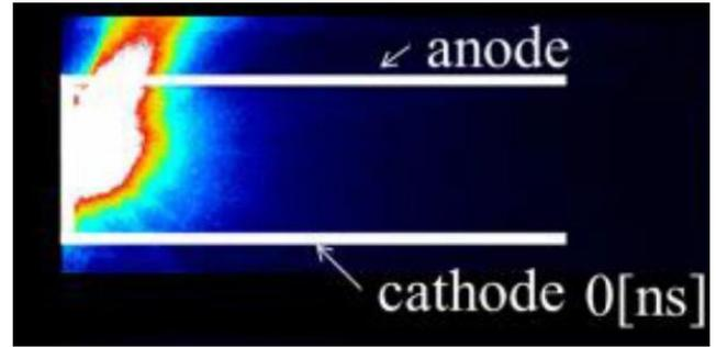
Figure 7. A typically observation data of the plasma in a LA-PPT by the ICCD camera
