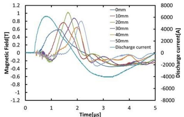
Figure 12. Output signals of magnetic field measured on center axis at 0 to 50 mm from propellant surface (charge voltage: 1,000V).
