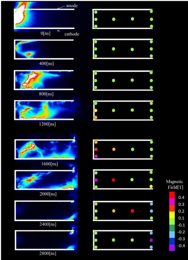
Figure 13. The light intensity of plasma, left and the magnetic fields in a LA-PPT channel, right. Therefore, the time division is 400us.
